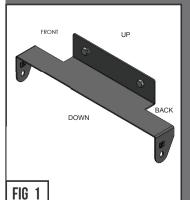
1) Begin by taking the ZROADZ Brackets and note where the ZROADZ Bracket mounting slots are located and that they will mount on the backside of front bumper.
